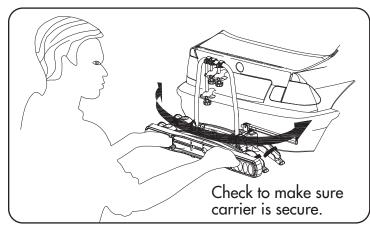
Tow ball bracket can be adjusted for a more secure fit.
